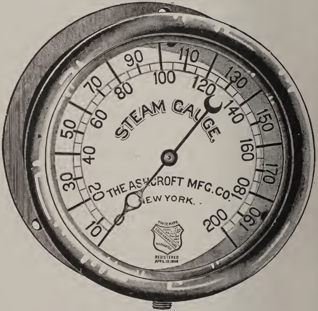
FIG. 73. AUXILIARY SPRING PRESSURE GAUGE.
